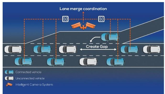
Fig. 1. Lane merge coordination of connected vehicles considering the behaviour of unconnected vehicles
