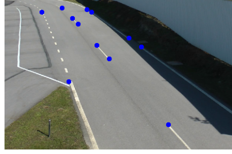
Figure 4: Visualization of 12 of the 15 landmarks used for the camera calibration.
